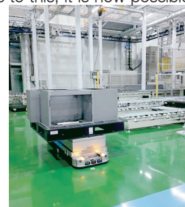
Autonomous mobile robots (AMR). They avoid people and obstacles and determine their own path of travel.
