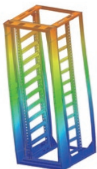
An example of vibration analysis (System rack)
